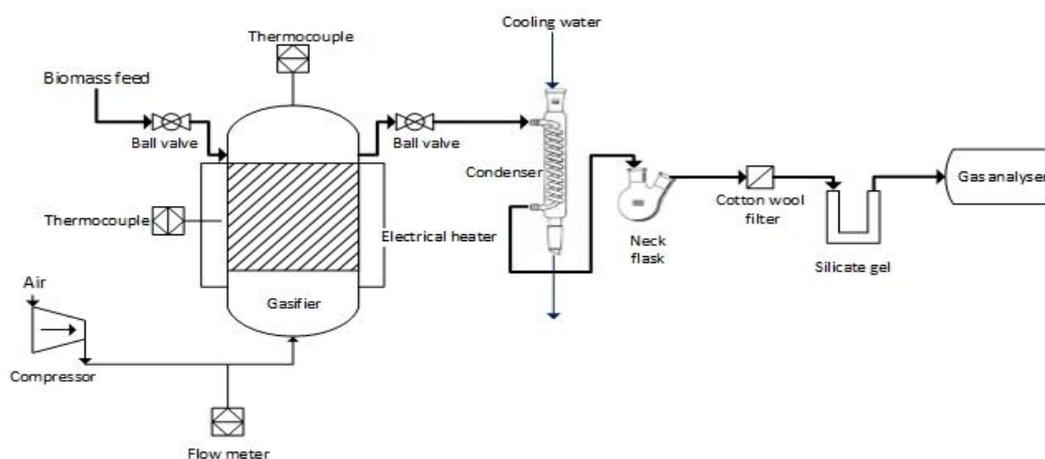
Figure 1: Schematic diagram of biomass air gasification in fluidised bed reactor
