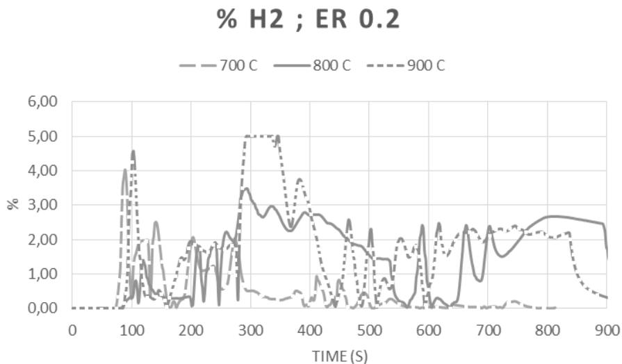
Figure 2: Real time H<sub>2</sub> composition of Oil palm Frond (OPF) at different temperatures
