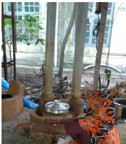
Figure 2: BUET single pot mud cooking stove and its isometric view within Autodesk Inventor
