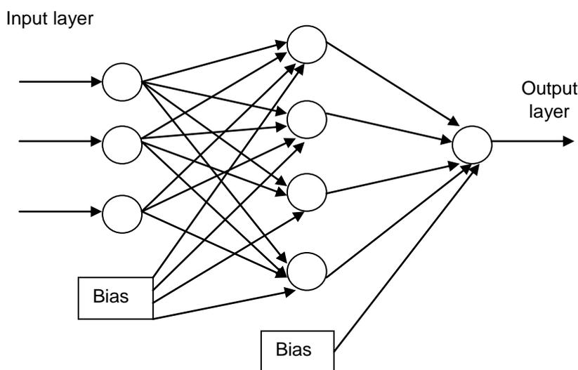
Figure 1: Schematics of a multi-layer artificial neural network.
