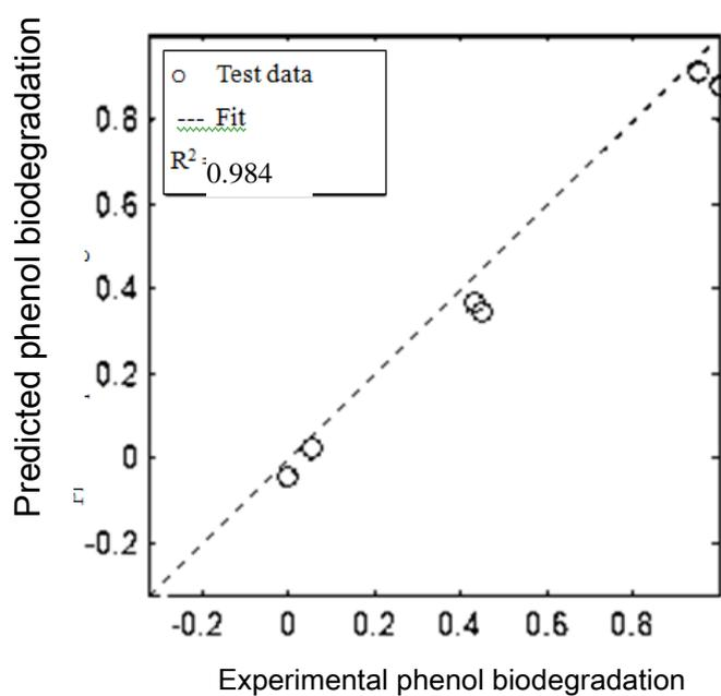
Figure 5: Correlation between estimated and experimental biodegradation for the test set data.
