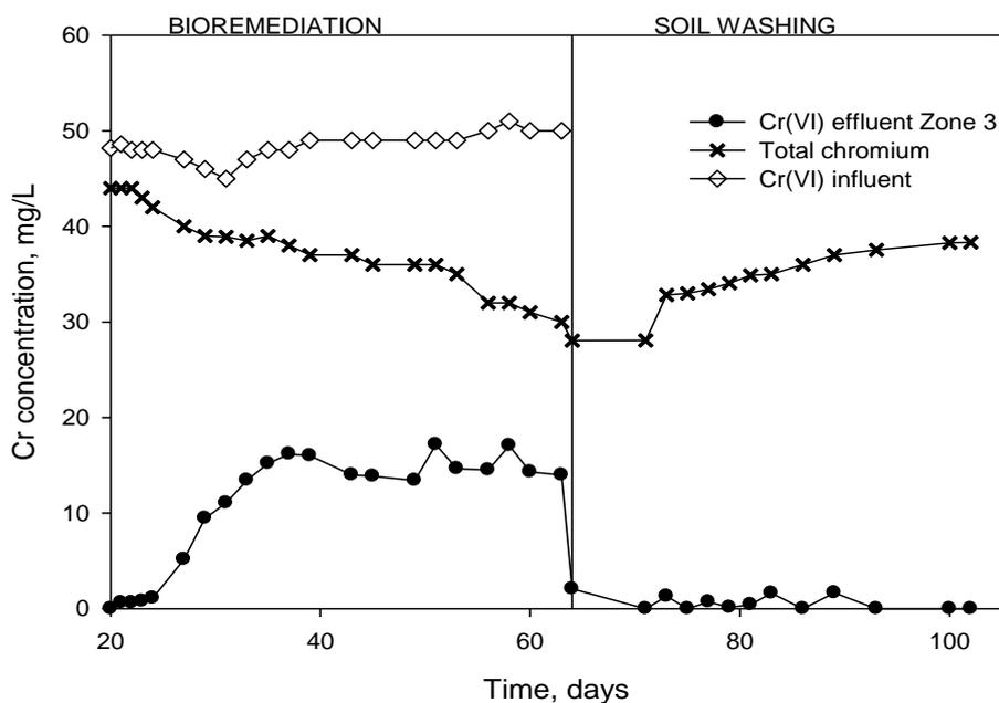
Figure 4: Cr(VI) and total Cr before and after the acid wash run showing an increase in total Cr in the effluent zone (Port 2) during the acid wash cycle.
