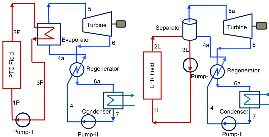
Figure 1: Simplified schematic of a PTC based CSP plant using regenerative ORC.
