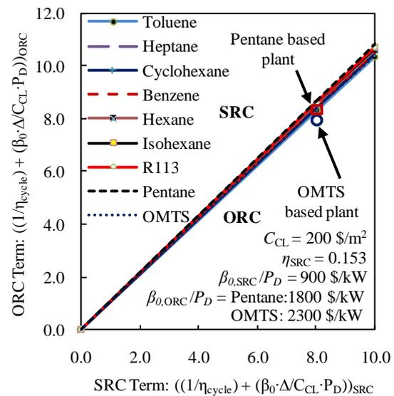
Figure 5. Variations in selection diagram with SRC efficiency (LFR based CSP plant).
