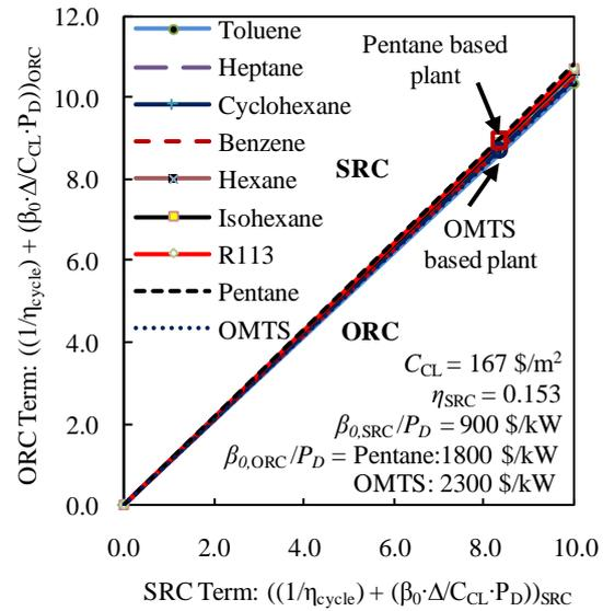
Figure 3: Selection diagram for SRC and ORC based plants (PTC based CSP plant).
