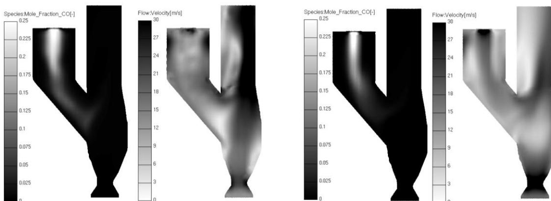
Figure 2: CO mole fraction and Velocity field: Only coal(left); Co-firing coal and plastic(right).
