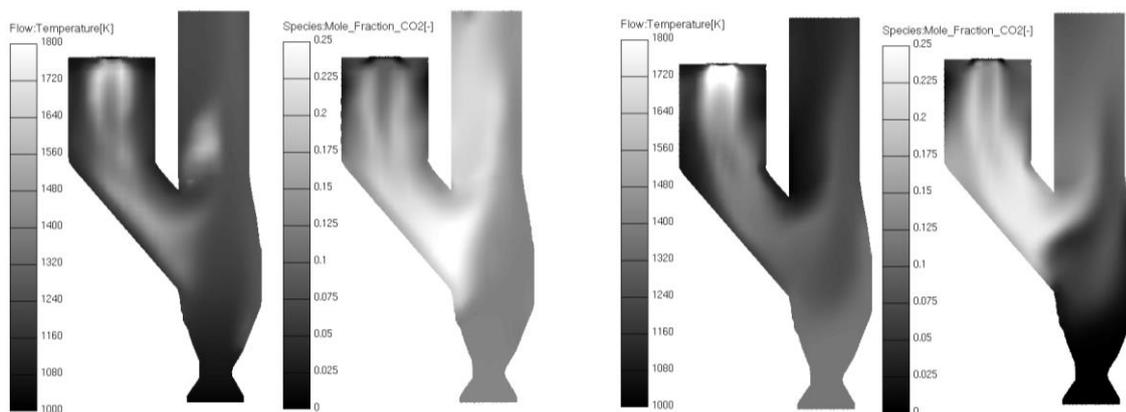
Figure 1: Temperature field and CO<sub>2</sub> mole fraction: Only coal(left); Co-firing coal and plastic(right).
