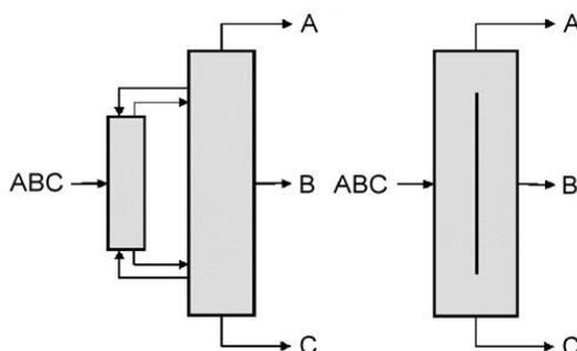
Figure 4: A middle-wall dividing wall column
