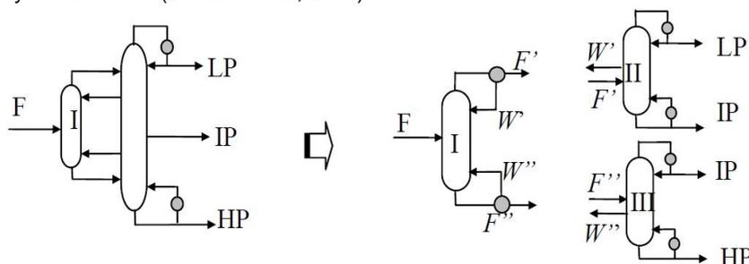
Figure 3: Thermodynamic equivalence of Petlyuk column
