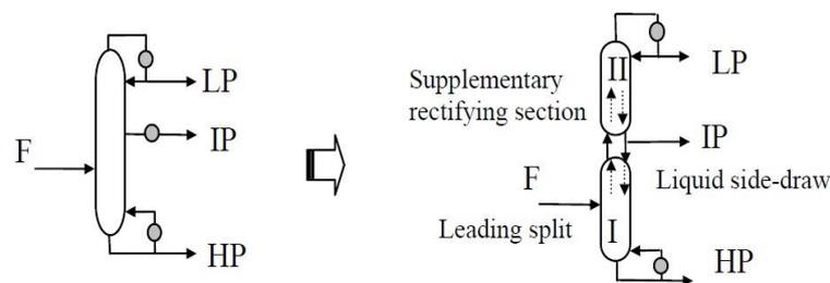
Figure 2: Thermodynamic equivalence of a liquid side-draw column
