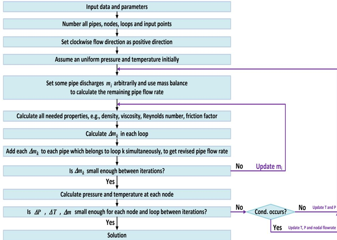
Figure 1: Procedures of steam network analysis
