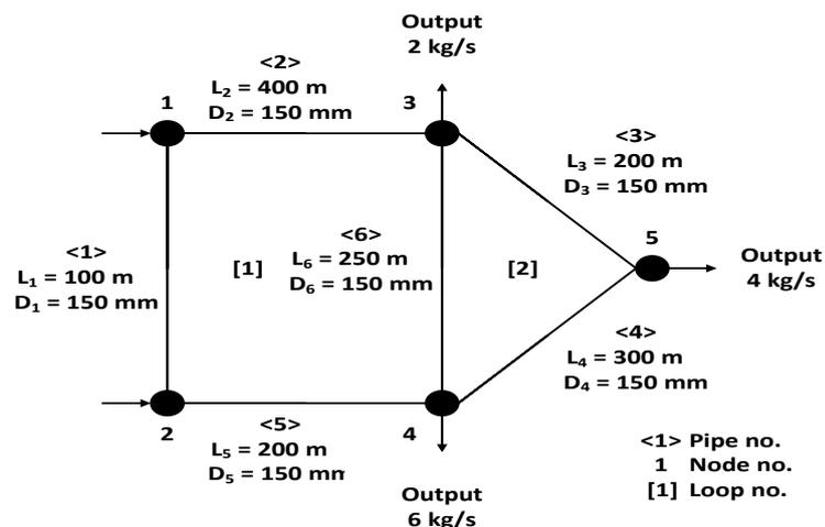
Figure 2: Layout of the network
