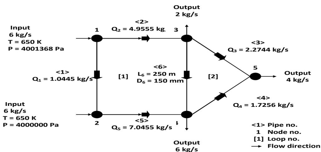
Figure 3: Flow pattern of the network
