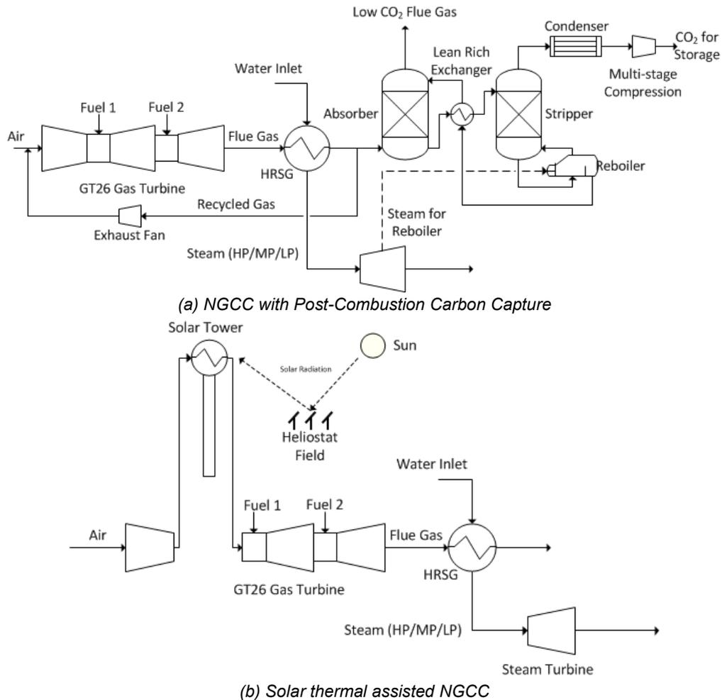
Figure 1: Basic process diagrams for the two processes studied, (a) NGCC power plant with solvent absorption post-combustion carbon capture, and (b) solar thermal assisted NGCC power plant
