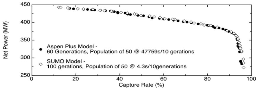
Figure 2: Comparison of the NGCC CCS plant surrogate model to the Aspen Plus® model. Number of generations and simulation CPU time is shown
