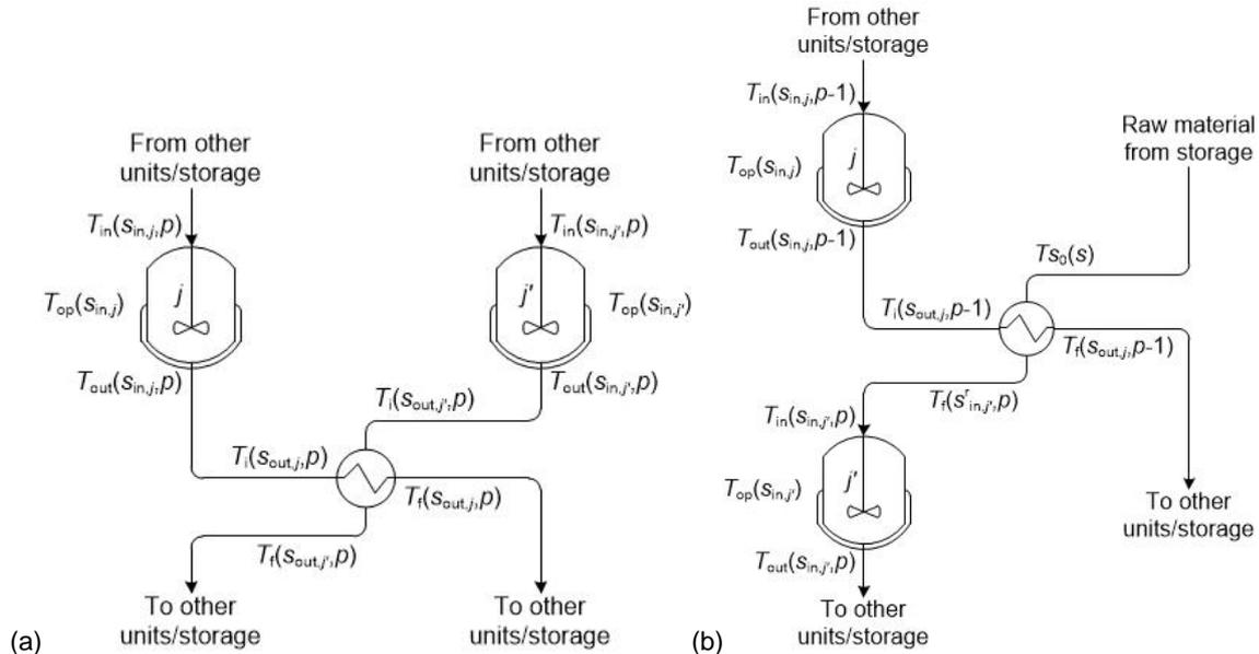
Figure 1: Superstructure for Heat Integration: (a) between outlet streams; (b) between outlet and raw material streams
