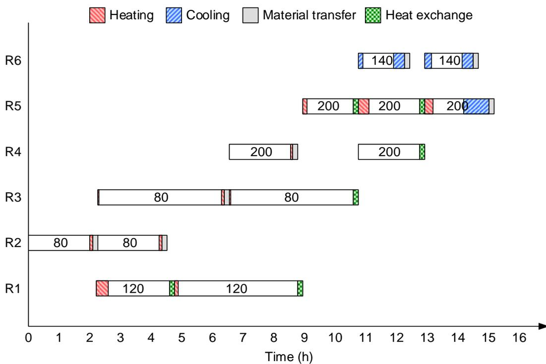
Figure 4: Optimal schedule with heat exchange among raw material and output streams
