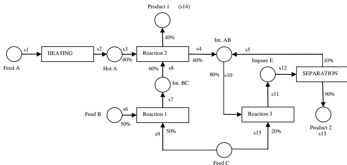
Figure 1: Flow sheet corresponding to the two-product batch plant.
