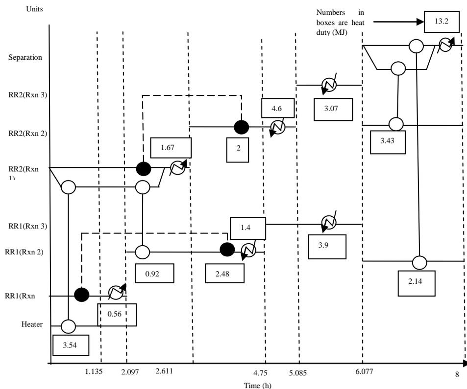
Figure 3: Possible HEN for Example 3 (heat exchangers with dotted line indicate heat exchange through intermediate fluid; the numbers in boxes represent heat duty in MJ)
