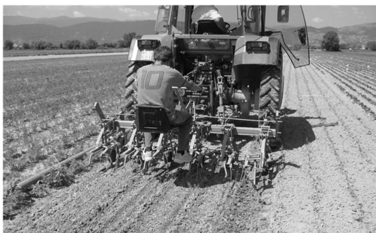
*Figure 3: Precision hoe at work in fennel*
