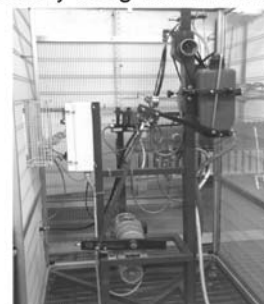
Hand-Held sprayer testing apparatus analysis according to UNI ISO 12100:2010
