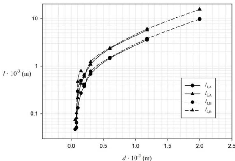
Figure 3: Critical thicknesses of ash deposit ( $l_1$  and  $l_2$ ) with respect to the particles' diameter
