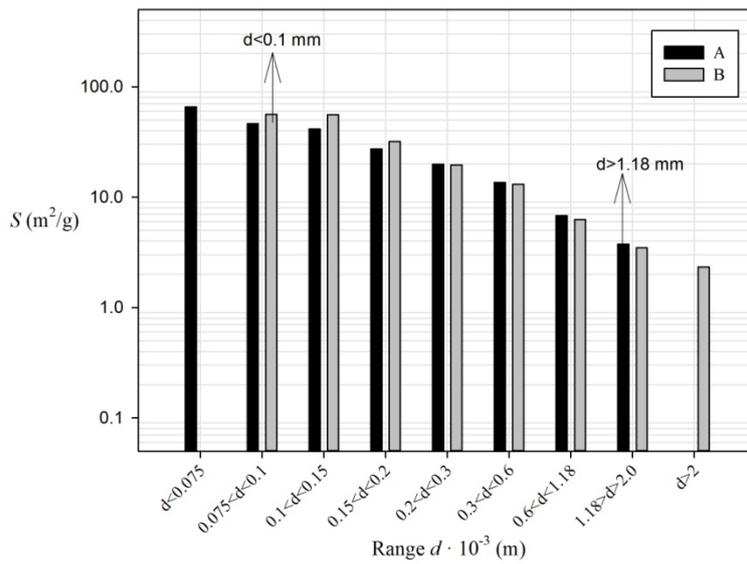
Figure 1: Specific surface area of samples with respect to the class of particles' size
