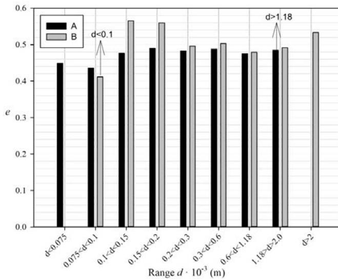
Figure 2: Voidage of samples with respect to the class of particles' size
