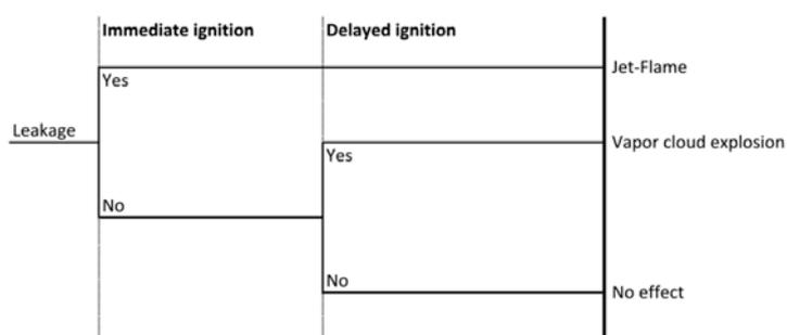
Figure 3: Event tree for biogas leakage event
