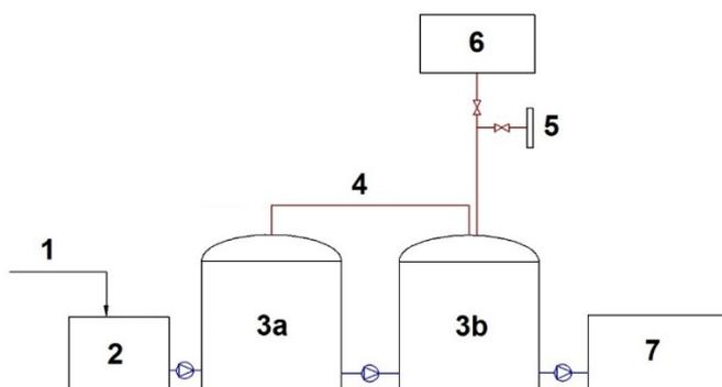
Figure 1: Basic technological scheme of wet-process biogas station
