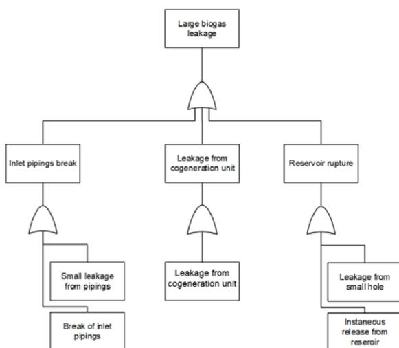
Figure 2: Fault tree for biogas leakage event
