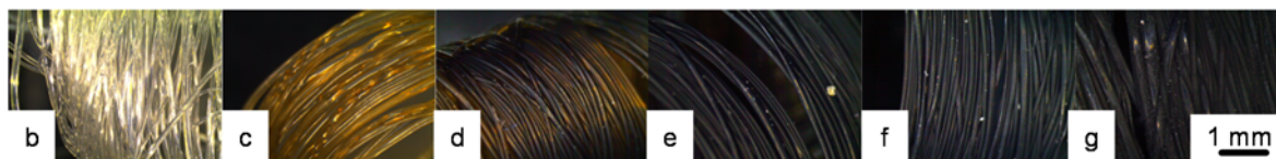
Figure 4: Colour change of the sulfonated HDPE fibres
