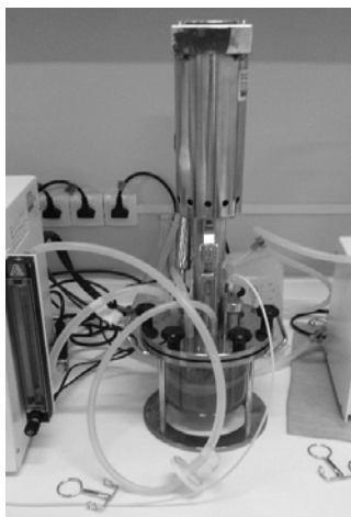
Figure 1: Bioreactor 1.2 l in a middle of a fermentation linked with the controllers
