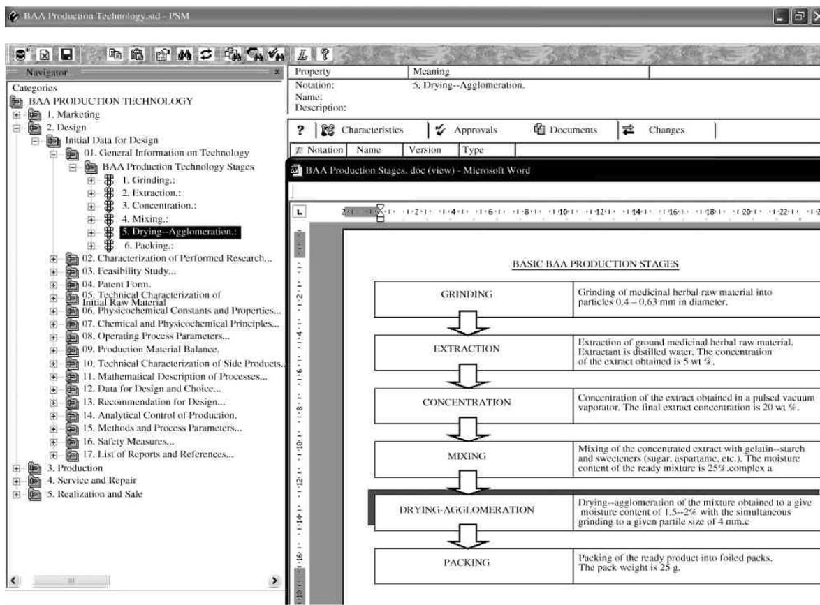
Figure 1: CALS Project element at the design step (basic stages of the technology of biologically active additives).
