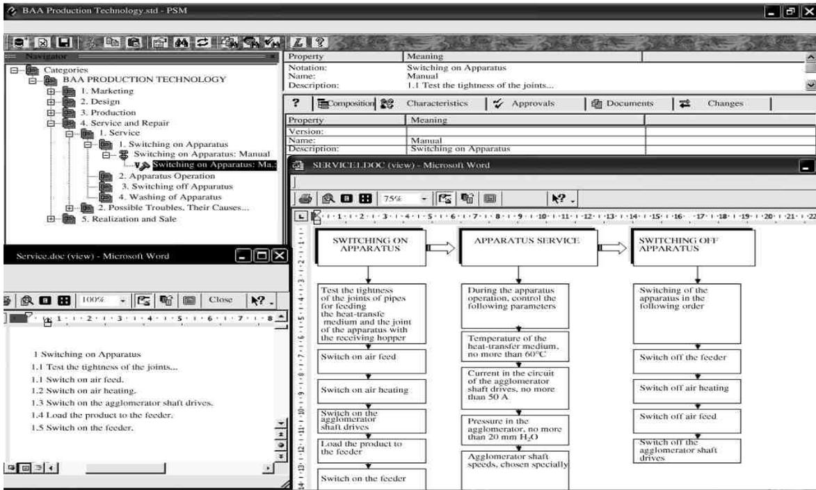
Figure 4: CALS Project element at the step of service of the dryer-agglomerator.
