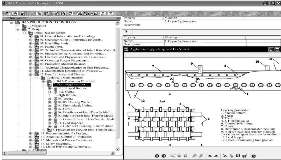
Figure 2: CALS Project element at the design step (dryer-agglomerator design).
