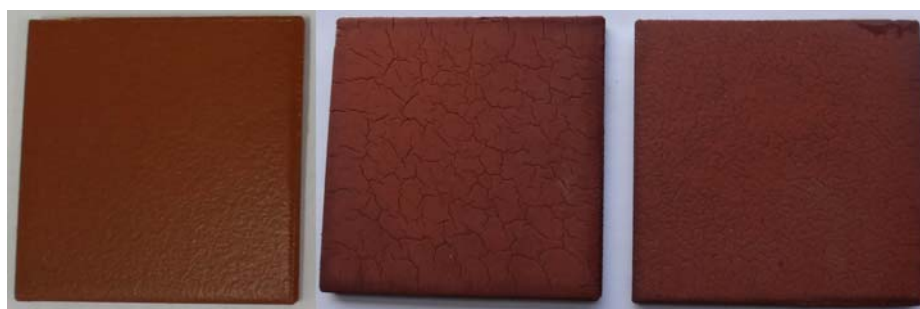
Figure 1: Discoloration and checking effect after 6 weeks UV exposure; a) Coat 2 specimen as painted, b) Coat2-(A) with ASTM 3 shrinkage checking and c) Coat2-(B) with ASTM 2 shrinkage checking.
