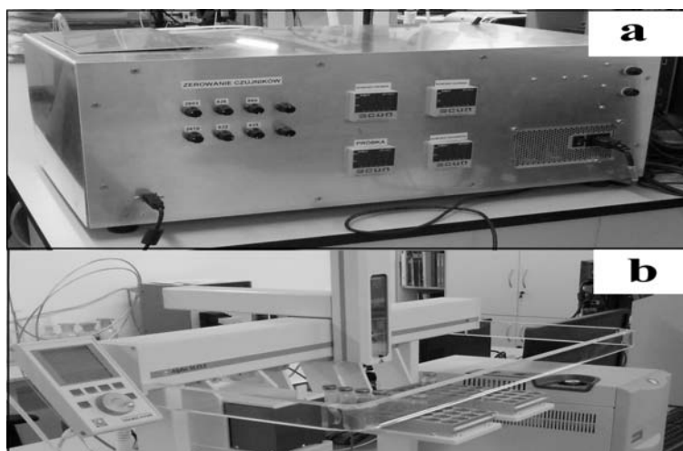
Figure 3: Prototype of electronic nose -(a), HERACLES II electronic nose of Fast/Flash GC type -(b).
