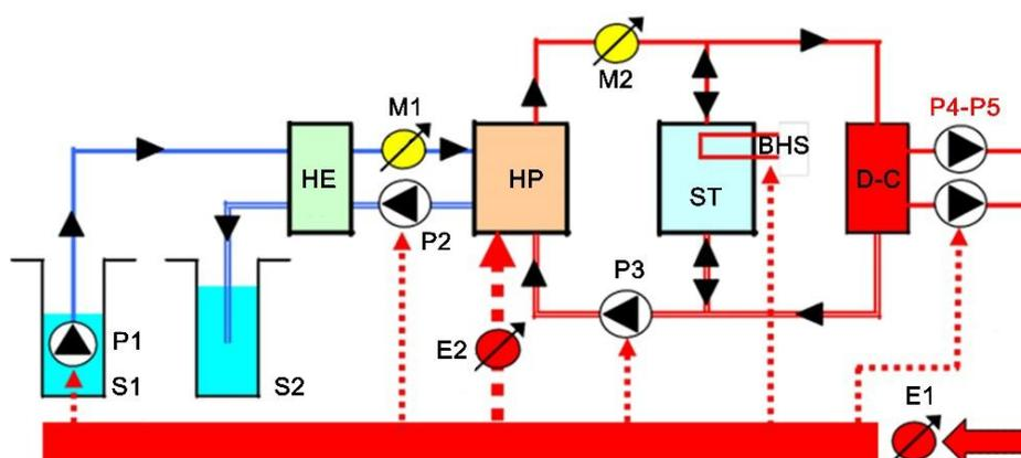
Figure 3: Depicted scheme of the connection of a heat pump water/water and electricity consumption
