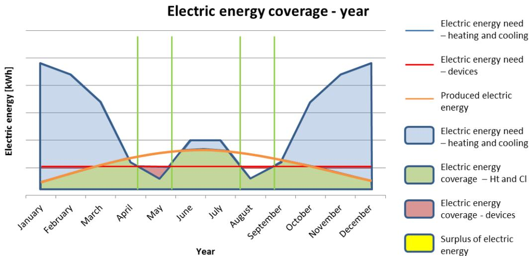
Figure 2: Electric power needs for heating, cooling, electricity and produced electricity by PV system during the year
