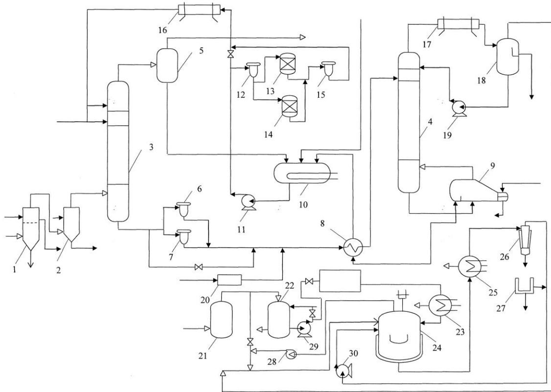
Figure 1: Technological scheme for ammonium bicarbonate based carbon dioxide utilization
