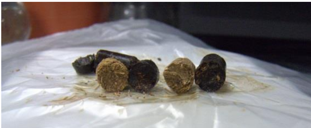
Figure 2: Palm pellet (light brown – left) vs. Energy Pack (dark brown – right) – after waste engine oil absorption to inner layer of pellet
