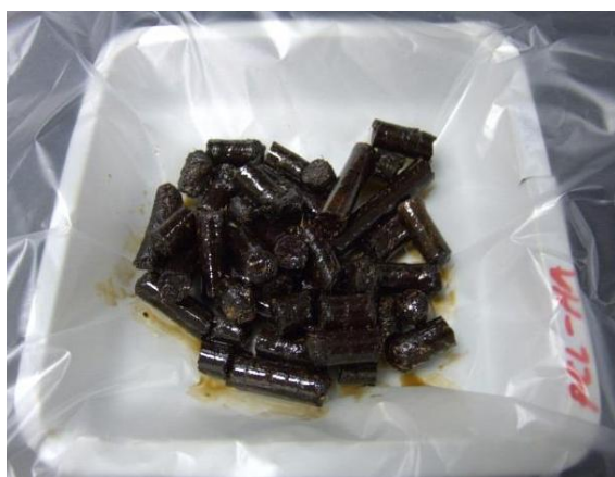
Figure 3(b): Energy Pack – palm pellet after waste oil absorption
