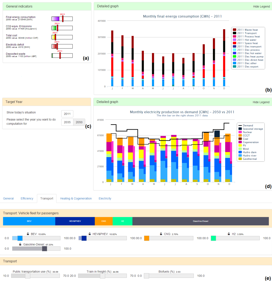
Figure 2: Screenshots of the Swiss-EnergyScope.ch calculator: (a) “General Indicators” showing calculations output KPIs, (c) “Target Year” for calculation year choice, (b) “Detailed graph” showing the 2011 final energy consumption and (d) a possible projection for 2050 electricity production (the black line on top of the bars representing the demand), (e) “Transport” input tab allowing for technologies selection
