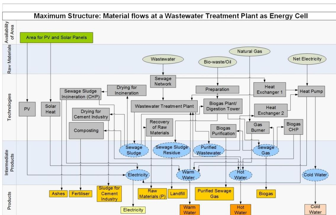
Figure 5: All possible material flows at a waste water treatment plant seen as an energy cell – first draft
