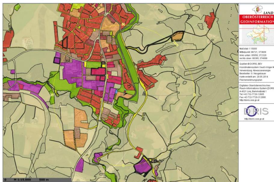
Figure 2: Sewage Plant, adapted map with different coloured development areas, potential heat consumers within 1 km circle are shown (created by Neugebauer G., 2014)
