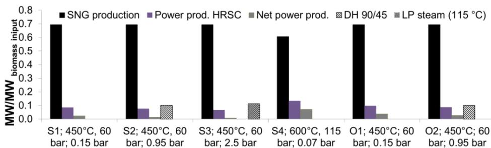
Figure 3: Conversion efficiencies for products in the SNG production system for cases with different operating parameters of the HRSC and biomass drying alternatives
