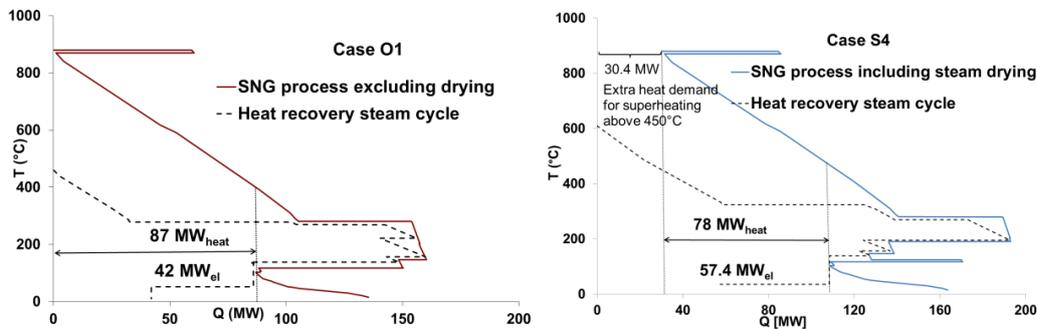
Figure 2: Left; split GCC for the SNG process (without biomass drying) and an HRSC. Right: split GCC for the SNG process with steam drying. Extra heat is used for superheating the steam in the HRSC
