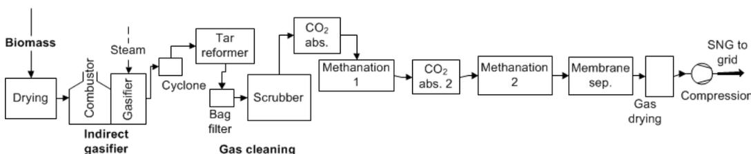
Figure 1: Flow sheet of biomass gasification based SNG production and final upgrading to grid quality
