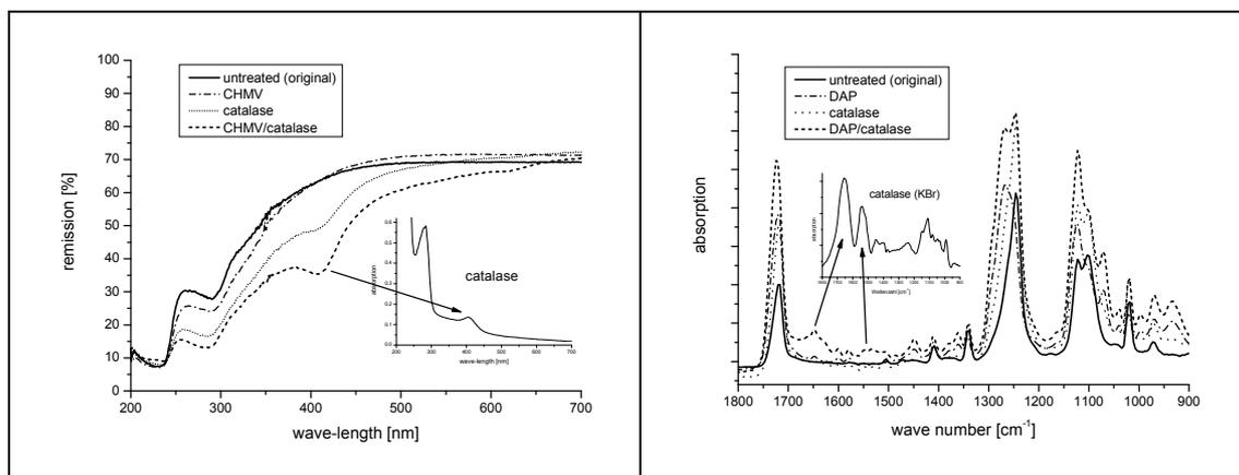
Figure 3: UV-Vis-spectra of PA 6.6 fabrics (left) and FT-IR(ATR)-spectra of PET fabrics (right) before and after UV-irradiation in the presence of the used cross-linker, catalase and both together (Opwis et al., 2005).
