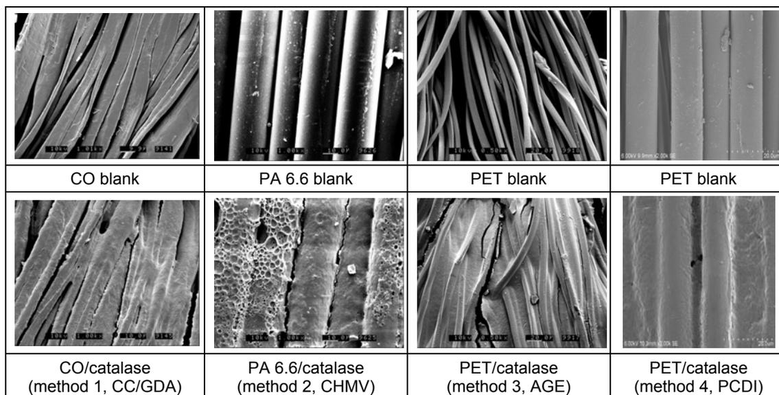
Figure 2: SEM of various textile carrier fabrics treated with catalase using different approaches (Opwis et al., 2004b, 2005, 2007, 2013).
