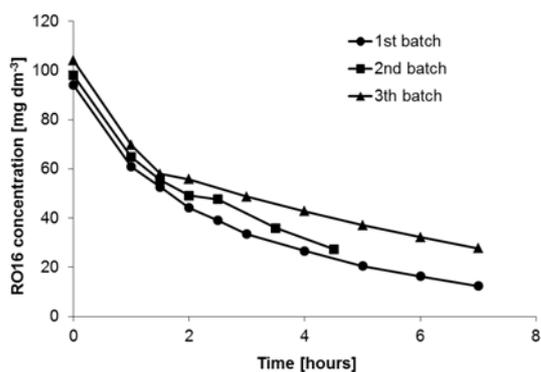
Figure 3: 1<sup>st</sup> set of batch decolorization experiments
