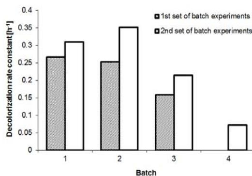
Figure 4: Decolorization rate constant for the dye RO16 in batch experiments
