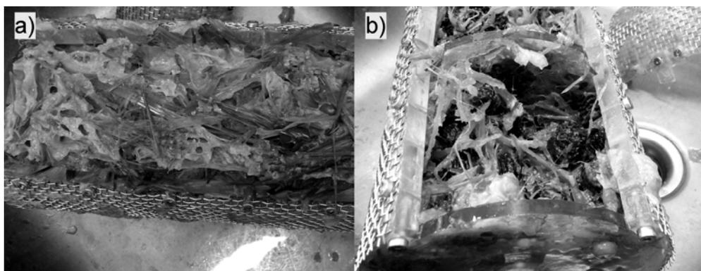
Figure 8: Snapshots of the inside of the drum of RDBC at the end of fungal cultivation
