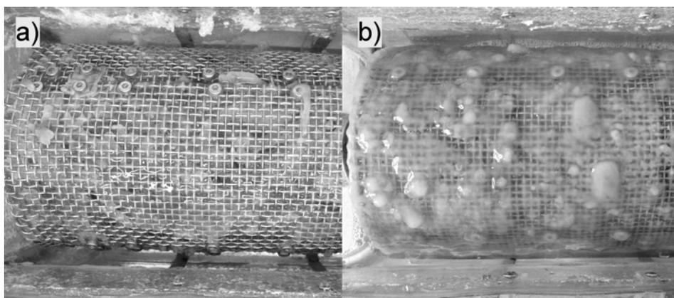
Figure 7: Snapshots of the drum in RDBC within 3<sup>rd</sup> continuous decolorization experiment (glucose added to inlet liquid stream: a) before start of the experiment, b) at the end of the experiment (after 25 days)
