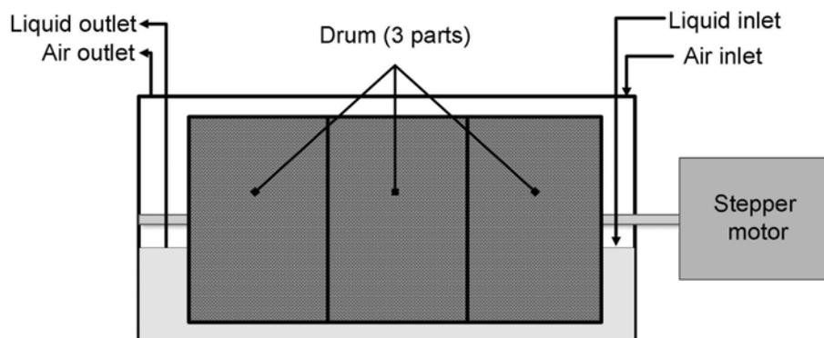
Figure 2: Schematics of the rotating drum biological contactor used in experiments
