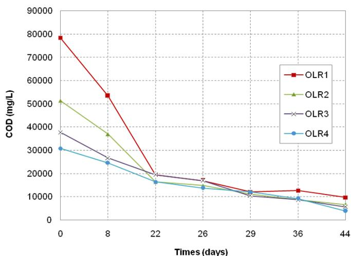
Figure 5: Variation of COD with time for different tested OLR
