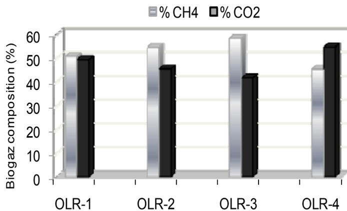
Figure 4: Biogas composition, (T=55 ° C)
