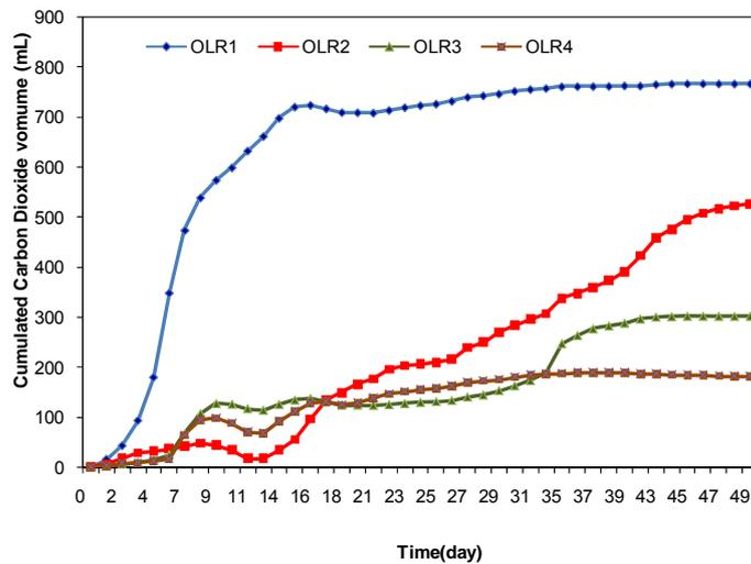
Figure 3: Cumulated CO<sub>2</sub> volume (T=55 ° C)
