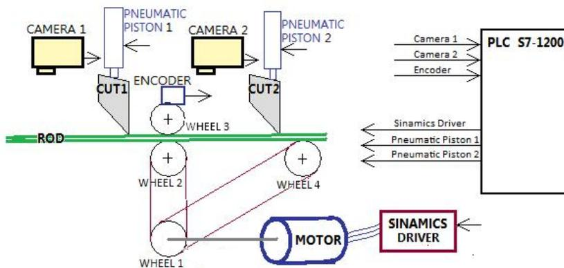
Figure 4. Block diagram of the measuring and cutting component
