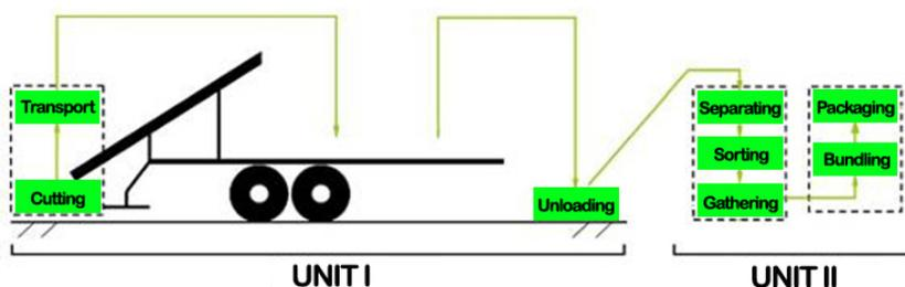
Figure 1. Rod Picker prototype concept
