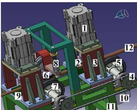
Figure 2. Measuring and Cutting Component Schematics: 1 - air cylinder for blade powering; 2 - blade and its support and guiding; 3 - cutting skeleton; 4 - rotary wheels for belt movement; 5,6,7 - rod guiding wheels (fixed and mobile); 8 - fixing spring; 9 - opposite blade ensemble; 10,11 - frame components; 12 - processed rod
