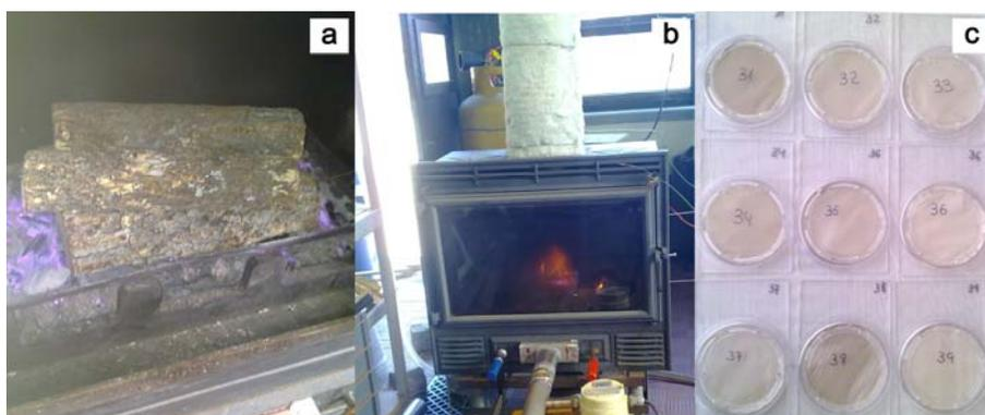
Figure 1: (a) detail of the wood logs in the combustion chamber, (b) view of the stove during combustion, and (c) filters for subsequent microscopy analysis
