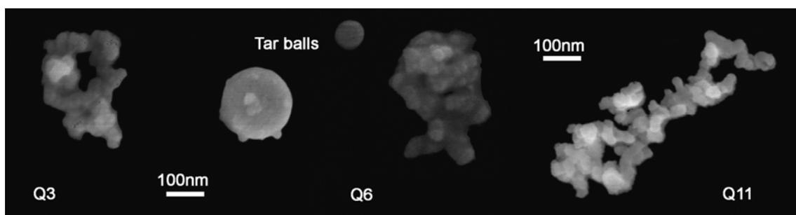
Figure 3: Examples of aggregates and tar balls in the samples from combustion experiments Q3, Q6 and Q11, respectively
