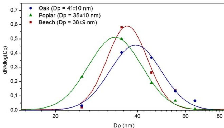
Figure 2: Lognormal curves of the size distributions of the monomers resulting from combustion of oak, poplar and beech experiments, respectively
