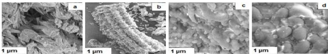
Figure 4: Scanning electron micrographs of (a) outer surface of RHA-6days, (b) skeleton of 2RHA-3days, (c) outer surface of RHA-3days (MCM-41), (d) outer surface of 2RHA-3days (MCM-48)
