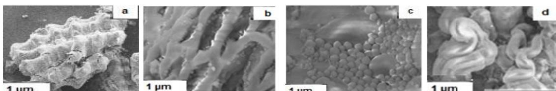
Figure 1: (a) Scanning electron micrographs of (a) skeleton of RHA-6days (MCM-41), (b) cross-section of the inner surface of RHA-6days, (c) outer surface of RHA-3days, (d) outer surface of RHA-6days
