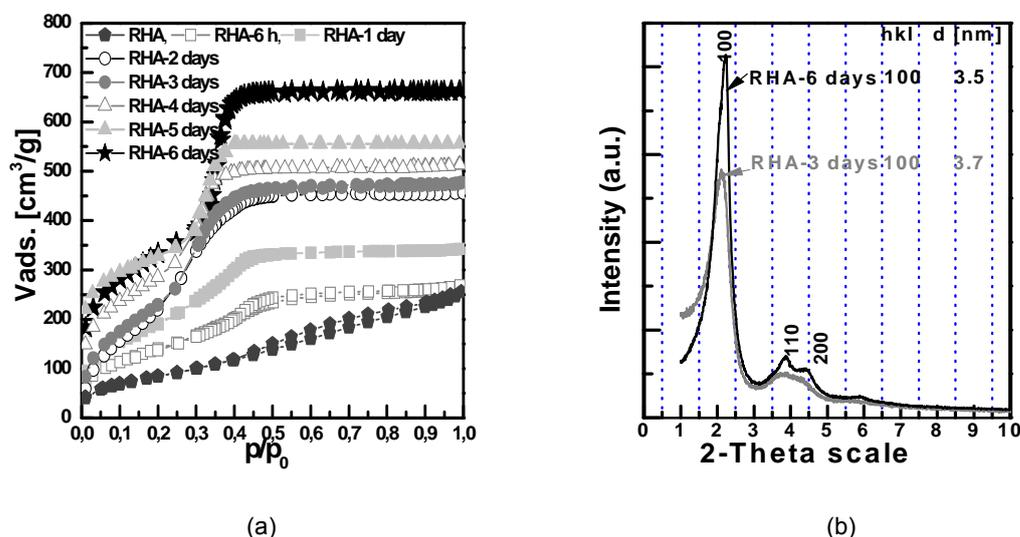
Figure 2: (a) Nitrogen sorption isotherms and (b) XRD patterns after pseudomorphic transformation of rice husk ash RHA into MCM-41 at different transformation times
