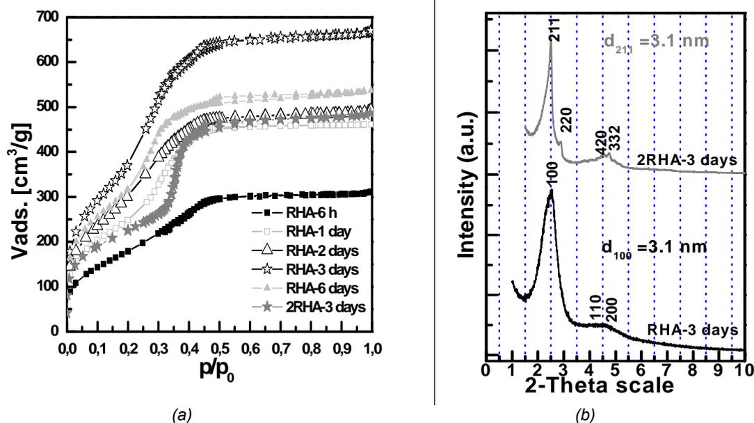
Figure 3: (a) Nitrogen sorption isotherms and (b) XRD patterns after pseudomorphic transformation of rice husk ash RHA into MCM-41 / MCM-48 at different transformation times
