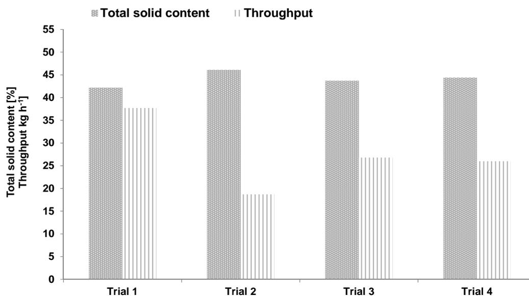
Figure 2: TS content and throughput of mechanical pre-treated BSG
