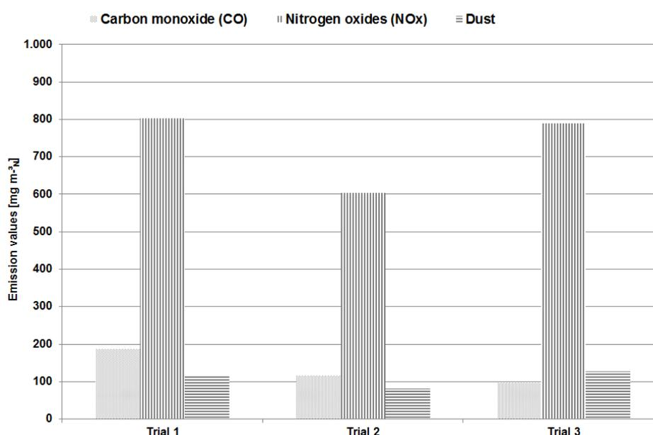
Figure 4: CO, NO<sub>x</sub> and dust emissions of the combustion trials
