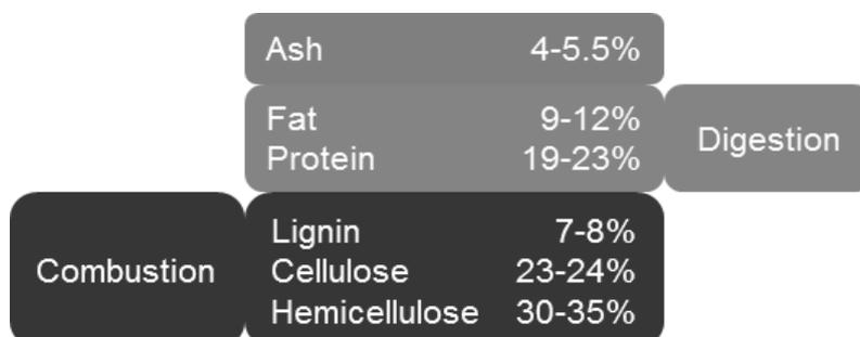
Figure 1: Chemical composition of BSG and optimal energetic usage (modified after Russ et al., 2005)
