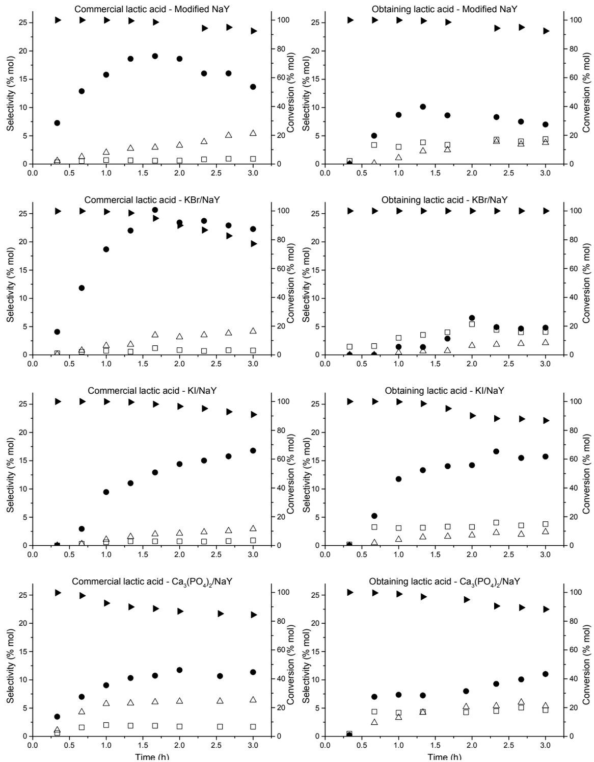
Figure 3. Results of the catalytic dehydration of commercial acid lactic and lactic acid obtaining by sugarcane molasses fermentation.  $\bullet$  acrylic acid,  $\blacktriangleright$  lactic acid,  $\Delta$  propionic acid
