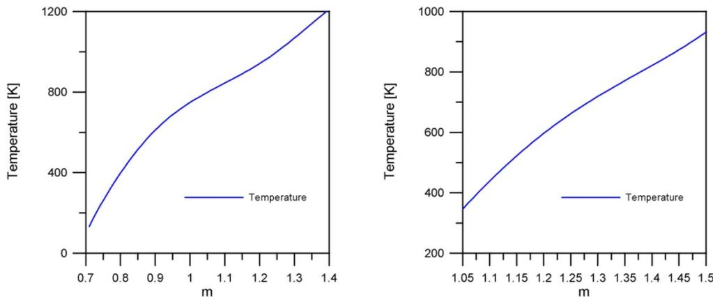
Figure 3. Gasification temperature for rice husk (left) and biosludge (right) as a function of the oxygen amount.
