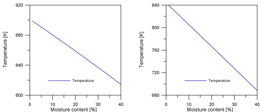
Figure 5. Effects of moisture content on gasification temperature for rice husk (left) and biosludge (right).
