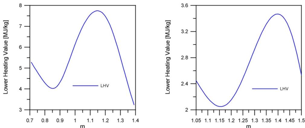
Figure 4. Syngas LHV for rice husk (left) and biosludge (right) as a function of the oxygen amount.
