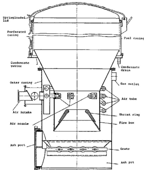
Figure 1. Scheme of the downdraft gasifier used in Taiwan.
