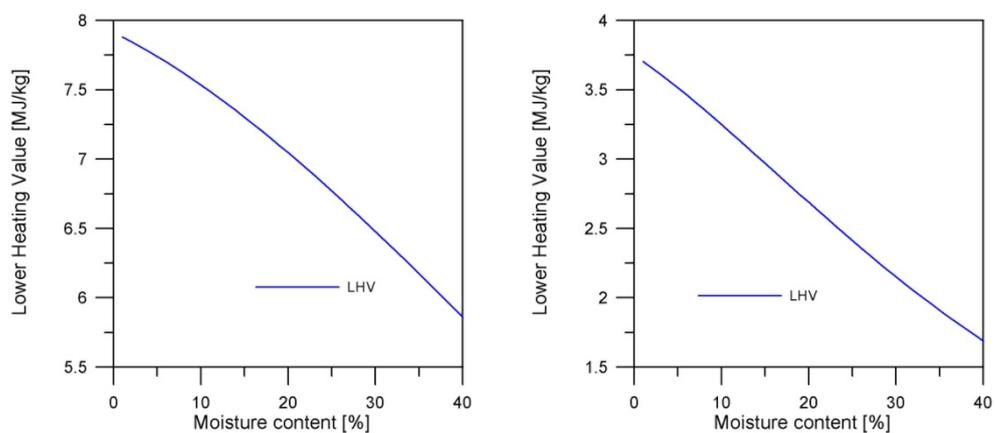
Figure 6. Effects of moisture content on the syngas LHV for rice husk (left) and biosludge (right).
