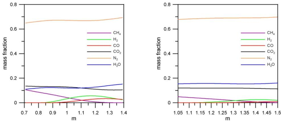
Figure 2. Syngas composition for rice husk (left) and biosludge (right) as a function of the oxygen amount.
