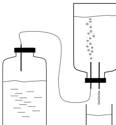
Figure 2: A simple apparatus for the measurement of biogas production by anaerobic fermentation using crimped vials. Left vial: fermentation vessel; right vial: gas collection vial
