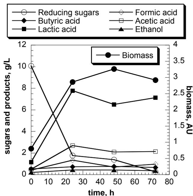
Figure 4: Time courses of reducing sugars, soluble fermentation products, and biomass concentrations during *Arundo donax* hydrolysate fermentation
