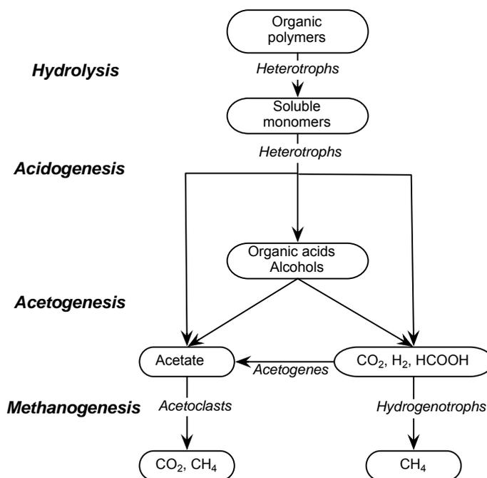
Figure 1: The anaerobic food chain (redrawn with modifications from Liu et al 2008).
