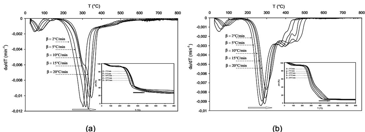
Figure 1. TG (inset) and DTG curves for rice straw under inert (0 % O<sub>2</sub>) (a) and oxidative (100 % O<sub>2</sub>) (b) atmospheres
