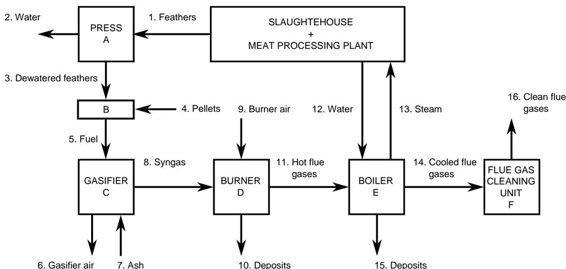
Figure 1: Schematic diagram of the Olsztyn gasification plant. Source: Kwiatkowski et al, 2013
