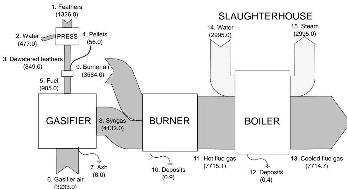
Figure 2 Sankey graph for the analysed gasification unit [kg/h]. Source: Kwiatkowski et al, 2013a
