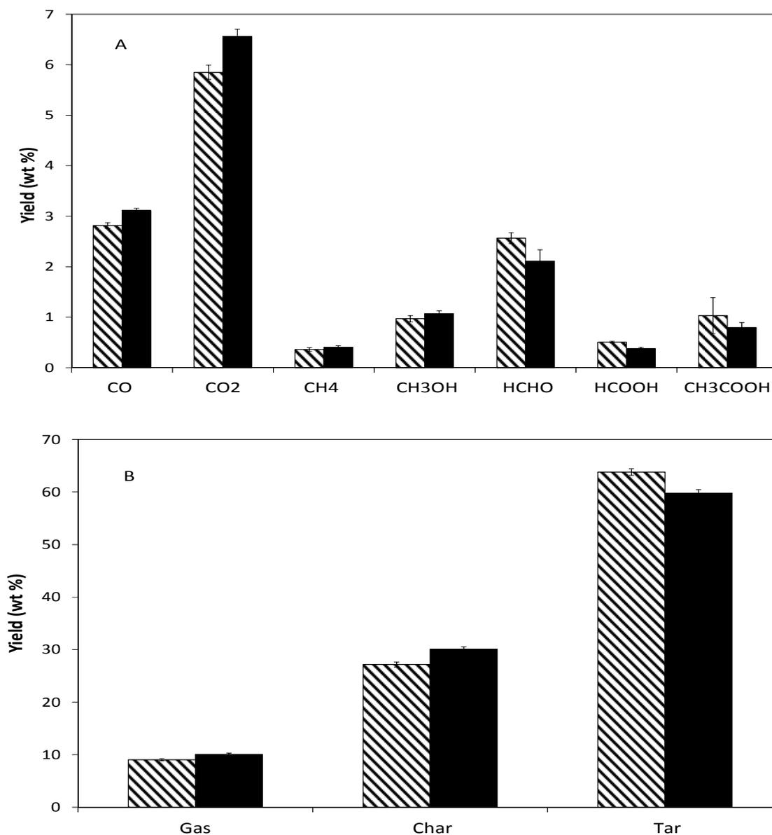
Figure 3 Representative yields of (A) individual species and (B) classes of compounds evolved during pyrolysis of cross-grain wood (cross-hatched bars), and parallel-grain wood (solid bars) at a nitrogen temperature of 418 °C. Error bars represent the standard deviations of three measurements.
