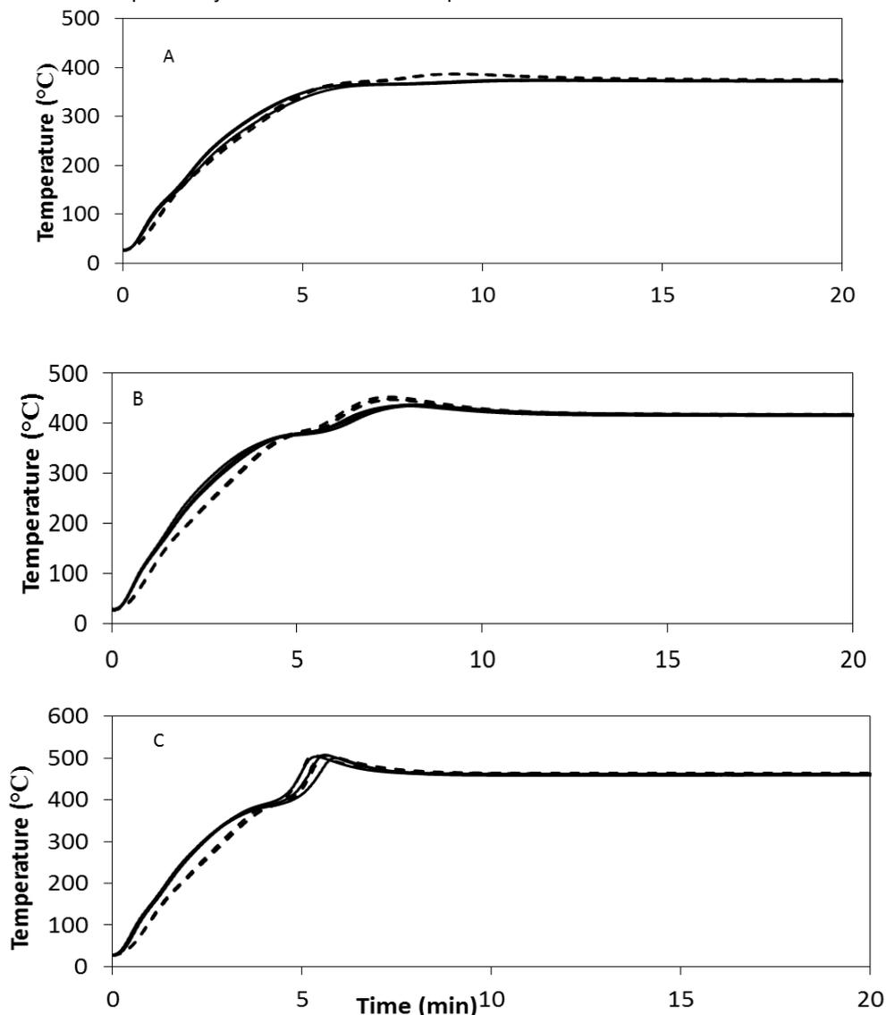
Figure 1: Temperatures measured at the center of the cylinder with nitrogen temperatures of 374 °C (A), 418 °C (B), and 464 °C (C). Solid lines represent experiments with cross-grain wood; dashed lines represent experiments with parallel-grain wood
