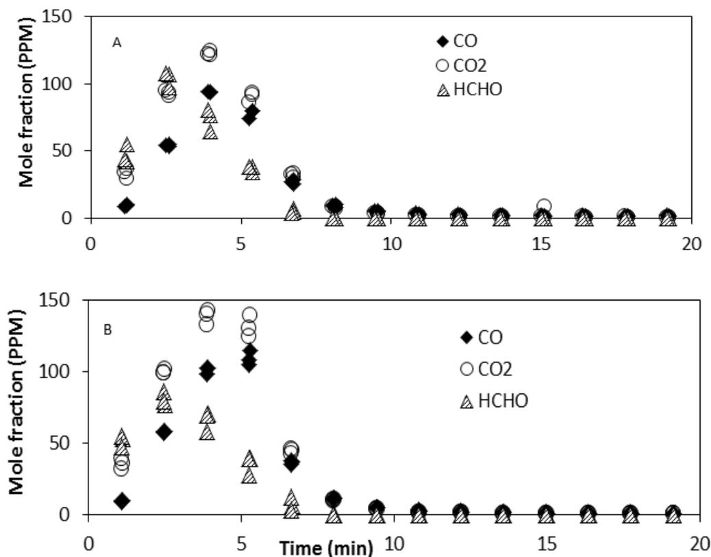
Figure 2: Representative time histories of species evolved during pyrolysis: Major species observed during pyrolysis of (A) cross-grain wood and (B) parallel-grain wood, with a nitrogen temperature of 418 °C
