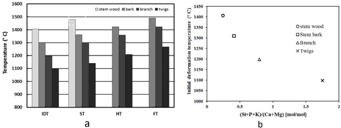
Figure 1: a) Ash fusion characteristic temperature of ashes from four parts of the spruce tree, b)
