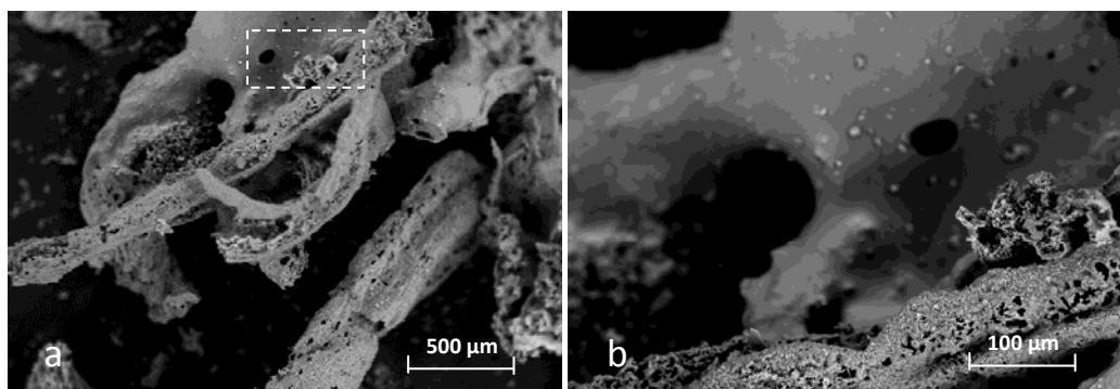
Figure 4: SEM image of twigs ash produced at 1000 °C
