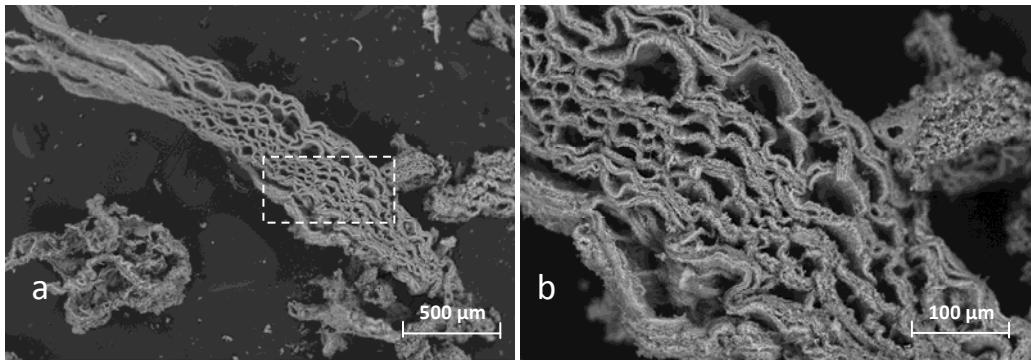
Figure 2: SEM image of stem wood ash produced at 1000 °C
