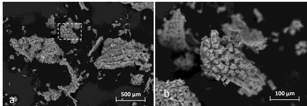
Figure 3: SEM image of stem bark ash produced at 1000 °C
