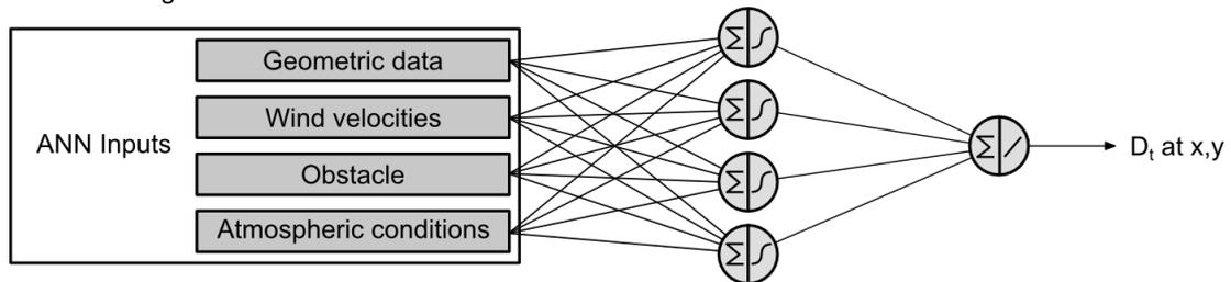
Figure 5: ANN inputs for  $D_t$  determination
