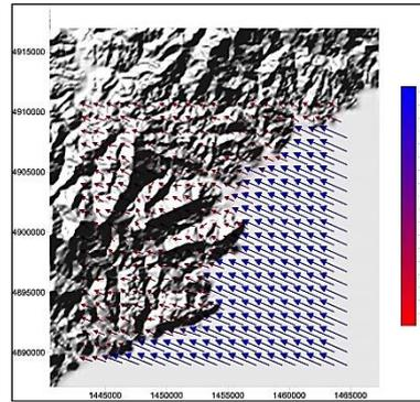
Figure 4: Three dimensional wind field simulation, performed by ADMS 5
