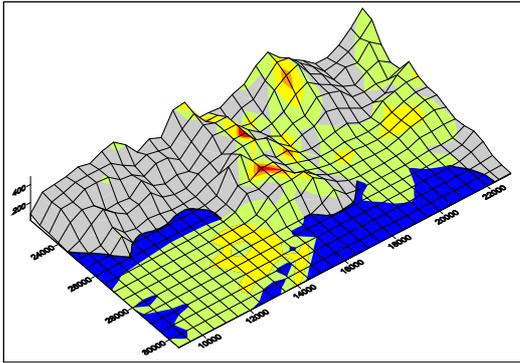
Figure 3: Ground level sulphur dioxide concentration modelling by SafeAirII
