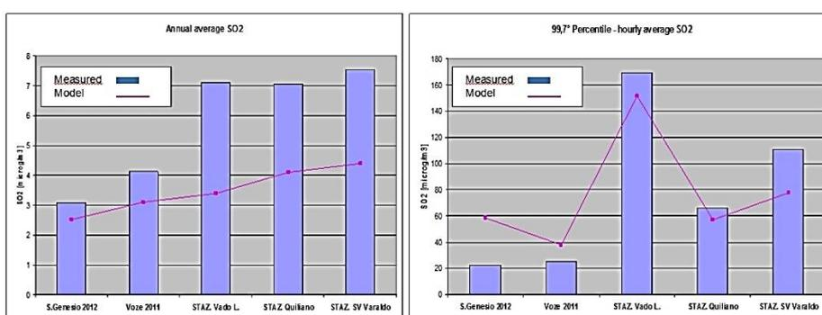
Figure 7: Comparison of calculated and measured concentration of the heuristic pollutant SO<sub>2</sub>
