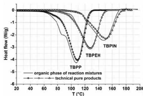
Figure 2: Non-isothermal DSC measurements, heating rate 5 K/min
