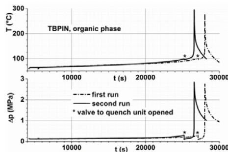
Figure 4: Adiabatic measurements of TBPIN, organic phase of reaction product
