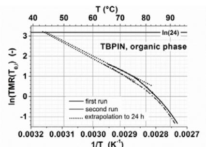
Figure 5:  $TMR_{ad24}$  derived from adiabatic measurements of TBPIN, organic phase of reaction product
