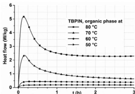
Figure 3: Isothermal TAM measurements of TBPIN, organic phase of reaction product
