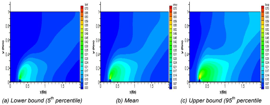
Figure 3: NO<sub>2</sub> plume dispersion for t= 1200 s
