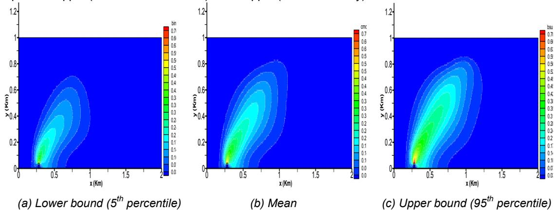
Figure 2: NO<sub>2</sub> plume dispersion for t = 100 s
