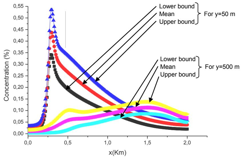
Figure 5: NO<sub>2</sub> plume dispersion at t= 1200 s, for fixed y
