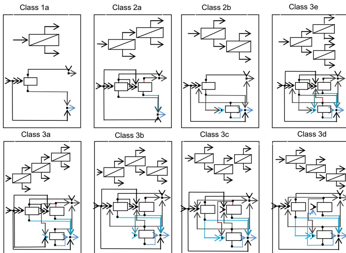
Figure 1: RO unit arrangements, and corresponding lean superstructures, for single unit, two-unit and three-unit design class options (Alnouri and Linke, 2012a).
