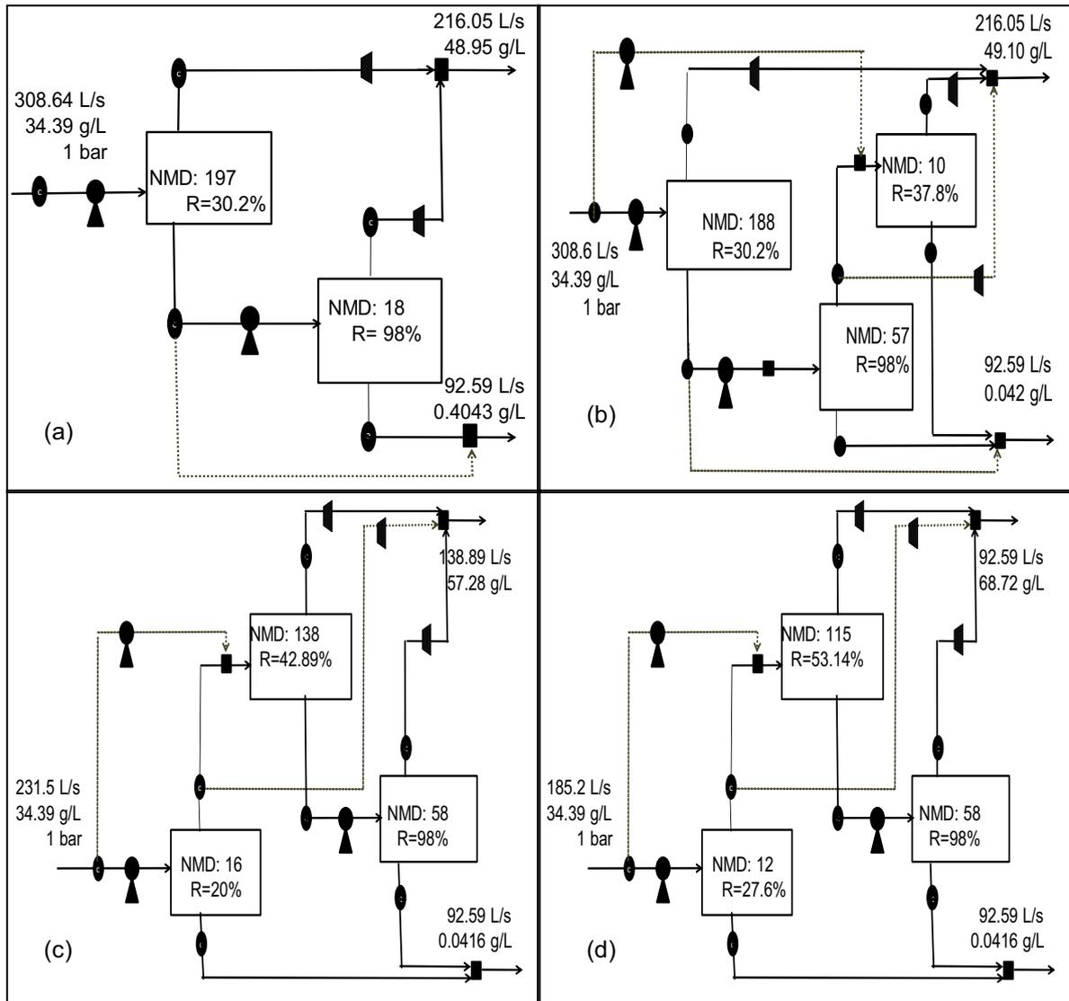
Figure 2: Summary of the best performing feasible design class solutions, for a Typical Seawater Feed case. (a)  $R=30\%$ , and 500 ppm water quality specification (b)  $R=30\%$ , and 150 ppm water quality specification, (c)  $R=40\%$ , and 150 ppm water quality specification, (d)  $R=50\%$ , and 150 ppm water quality specification
