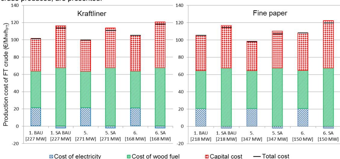
Figure 4: Specific production cost of FT crude (wood fuel 35 €/MWh; electricity 70 €/MWh).
