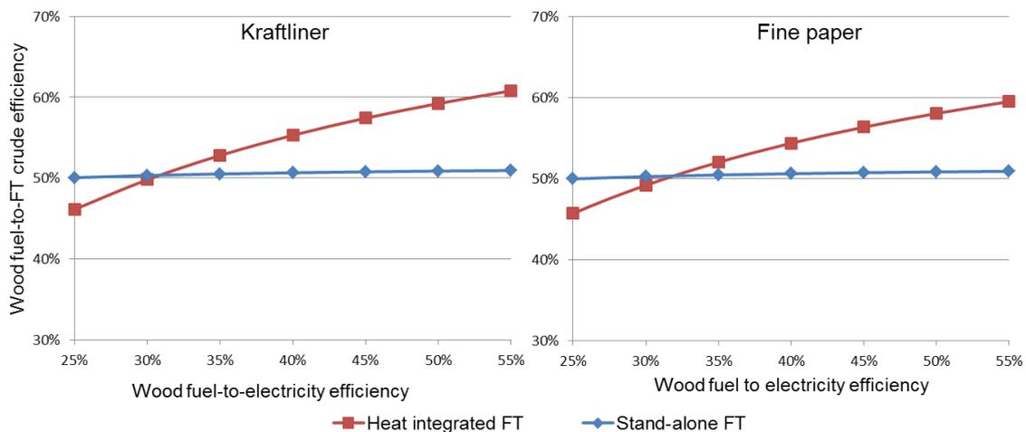
Figure 2: Wood fuel-to-FT crude efficiency. Electricity is valued as wood fuel, using varying wood fuel-to-electricity efficiencies
