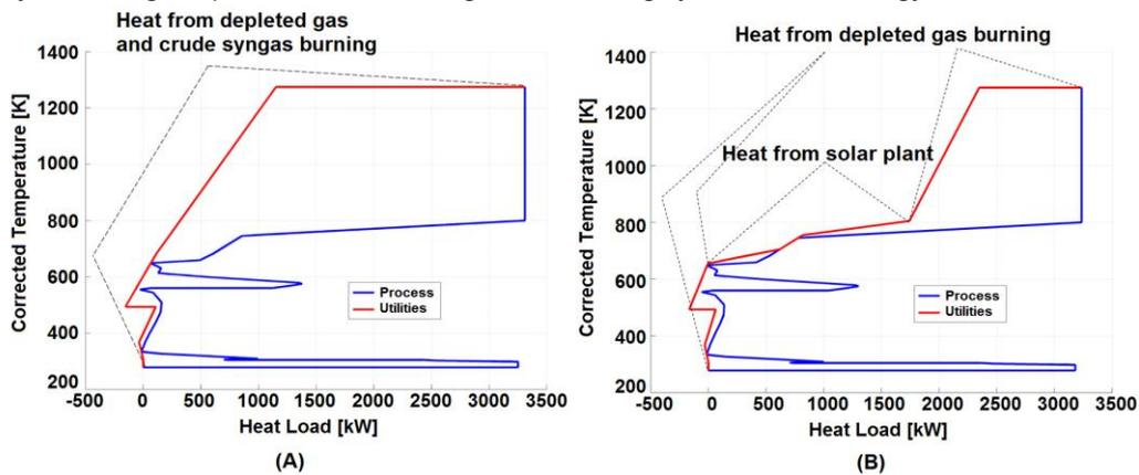
Figure 2: Heat load distribution of utilities and process streams without (A) and with (B) solar utility, in corrected temperature – heat load diagram
