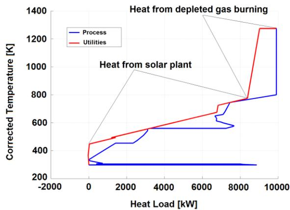
Figure 3: Heat load distribution of utilities and process streams with use of a heat recovery double pressure level Rankine cycle and hot air coming from a solar trough-receiver, output at 200 °C
