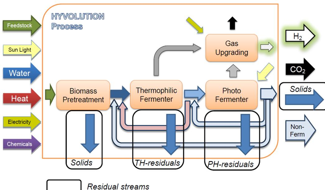
Figure 1: Scheme of HYVOLUTION process (Foglia et al., 2010)
