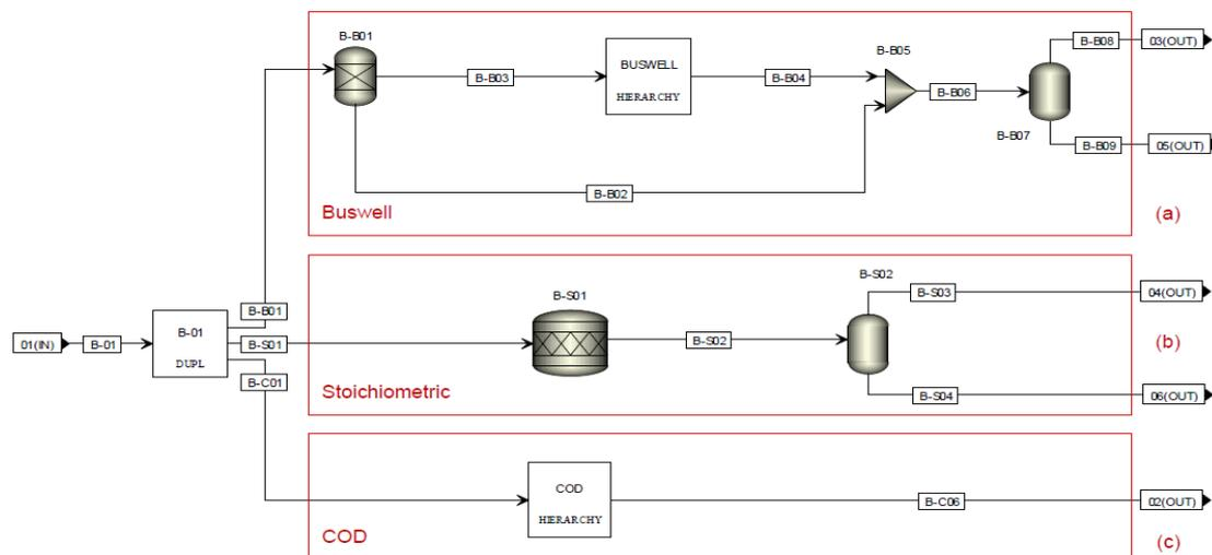
Figure 2: Biogas production routes in Aspen Plus
