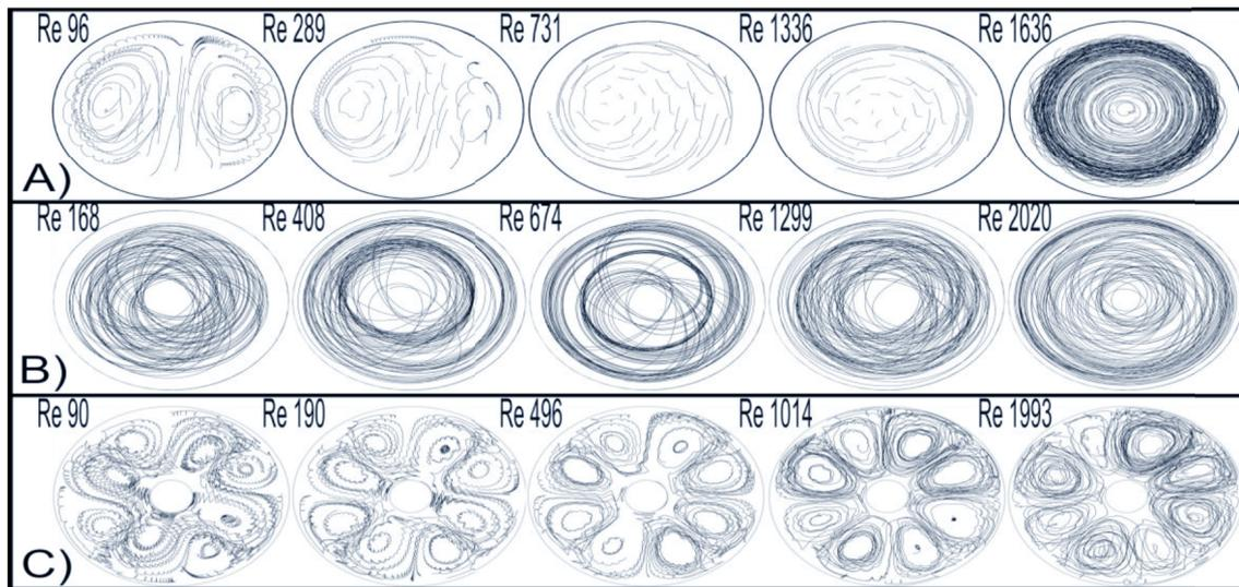
Figure 3: A) Coil insert flow patterns, B) twisted tape flow patterns and C) hiTRAN flow patterns
