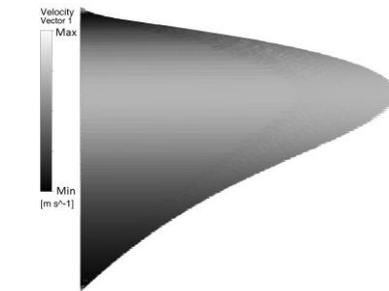
Figure 5: Mixed convection velocity profile, low velocity at bottom of tube and high velocity at top
