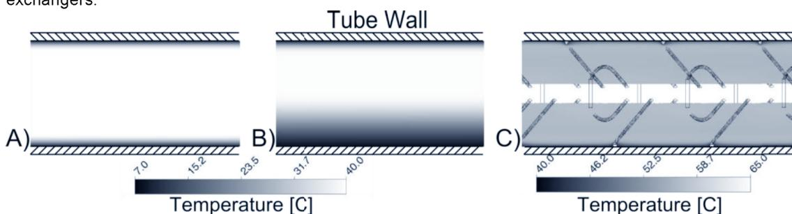
Figure 4: Temperature profile after 2500 mm a) empty tube in forced convection region, b) empty tube in mixed convection region and C) hiTRAN insert in mixed convection region
