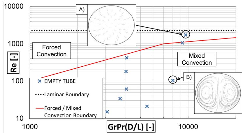
Figure 2: Forced and mixed convection regions, Metais and Eckert (1964). A) CFD forced convection flow patterns and B) CFD mixed convection flow patterns
