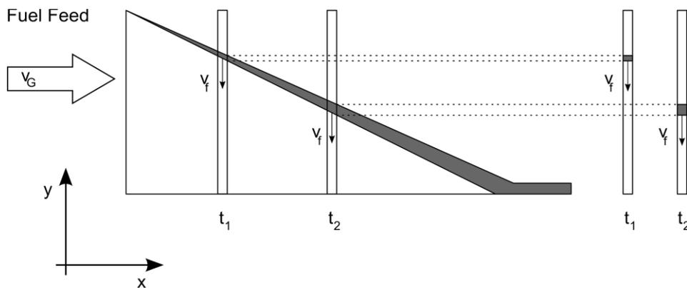
Figure 1: Walking column method. A fuel is moved on the grate with velocity  $v_G$ , so that horizontal position on the grate can be calculated using  $\Delta x = v_G \Delta t$ . As the combustion proceeds, the reaction front travels down with unknown velocity  $v_f$ .
